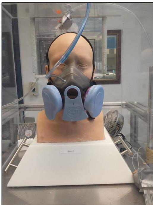
**Figure 48. HMER donned on medium static advanced headform.**
