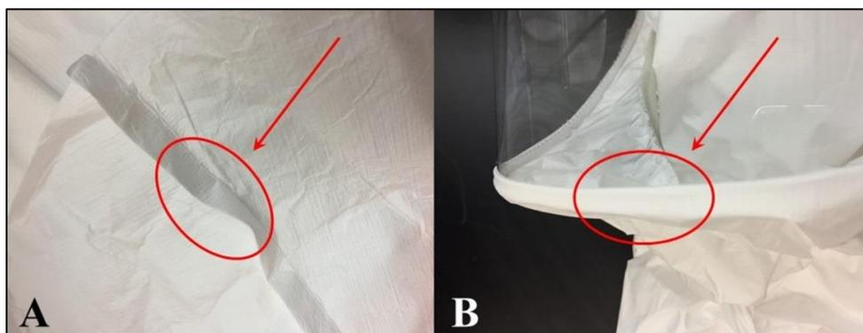
**Figure 50. A) Tychem-Tychem seam, B) Tychem-visor seam.**
