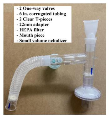
Filtered Aerosol Set-up
